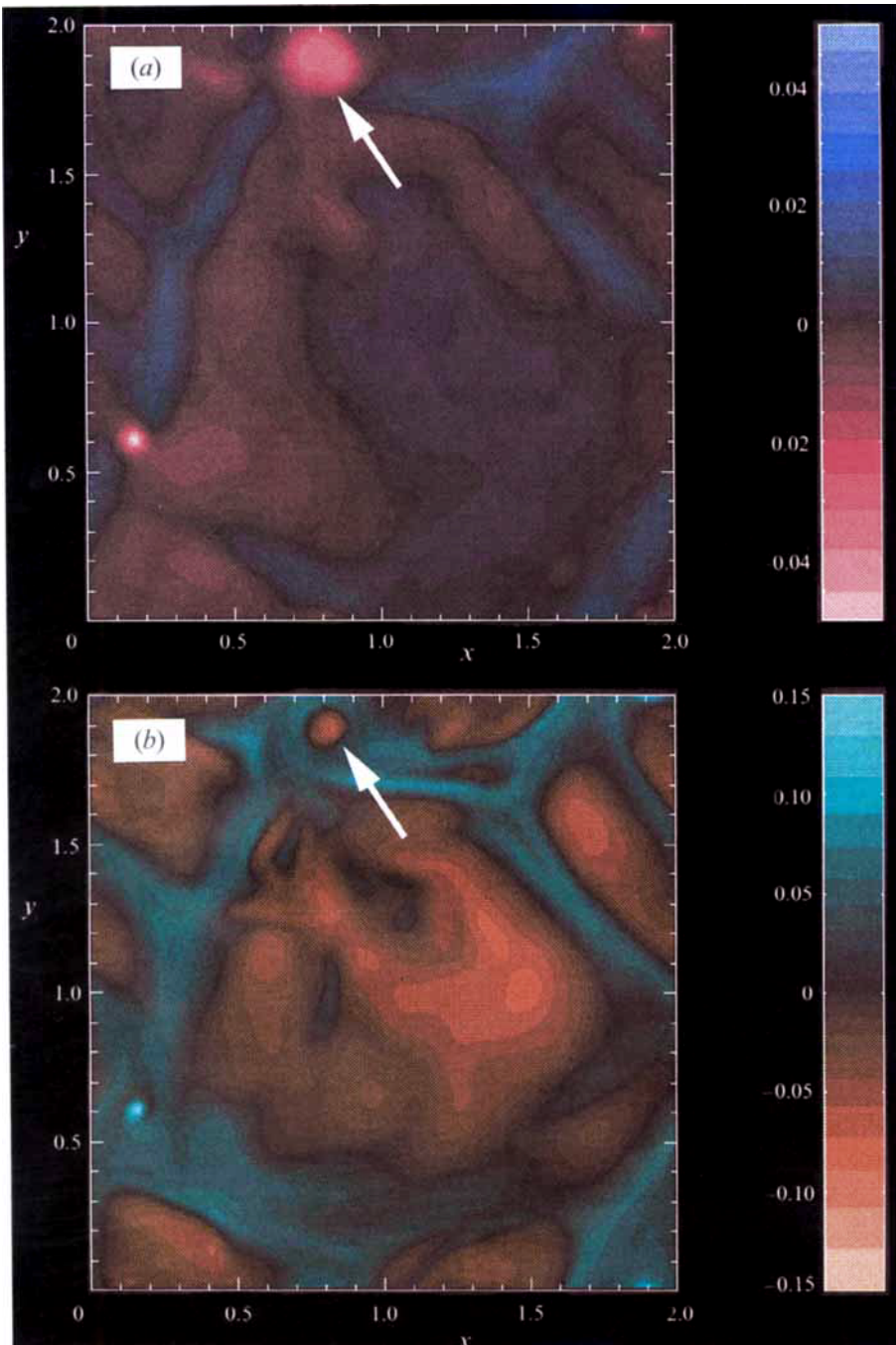
FIGURE 3. (a) Horizontal image of the relative density fluctuation \rho'/\rho . Light, low-density regions are pink. (b) Vertical velocity normalized by the sound speed, u_z/c . The arrows indicate a strong swirling downdraught where vortex buoyancy leads to an upward motion in the core of the vortex. Run D.
